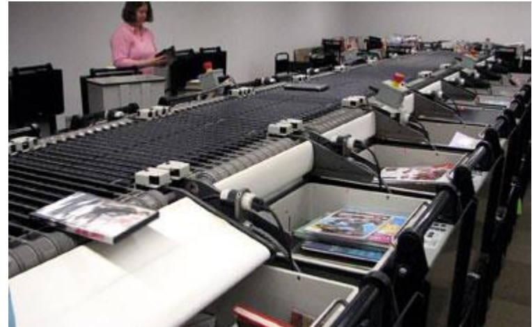
An automated materials handling system sorting books into bins, Champaign Public Library, Champaign, Illinois
