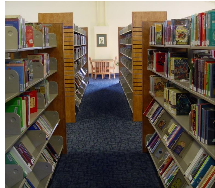
Tilting the bottom two shelves makes book spines easier to read & reach.
